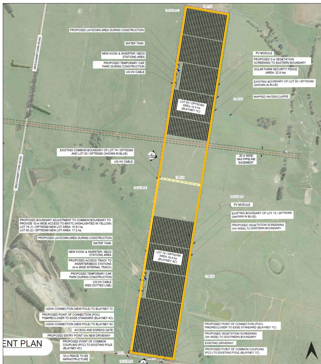
Figure 4 – Blayney 4C & 7C Solar and BESS project General Arrangement with APZ Highlighted
